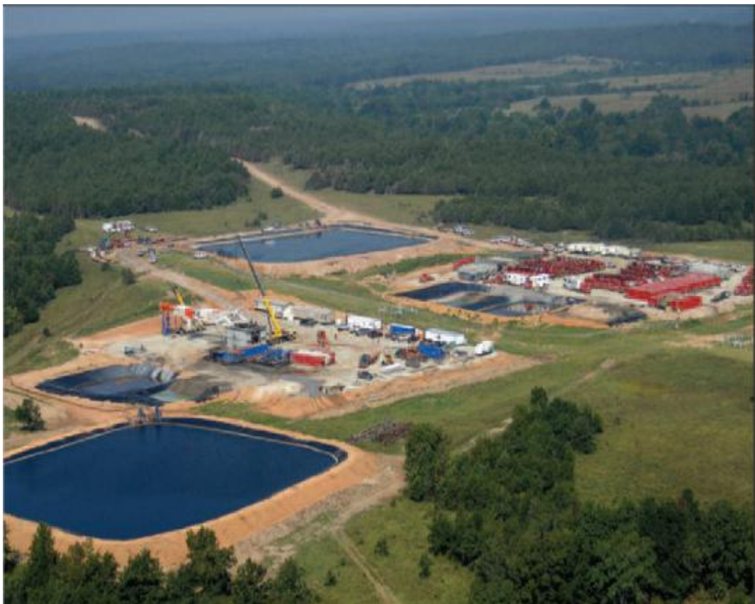
Figure 10: Frac Pits Adjacent to Drill Pads in Low Relief Terrain (Halliburton, 2008).
